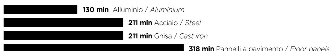
Messa a regime dei locali / Room heating capacity ( $5-21^{\circ}\text{C}$ ;  $\Delta t = 30^{\circ}\text{C}$ )
