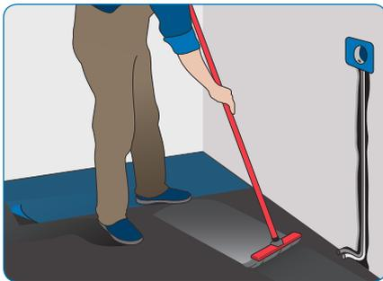
3) Cut out a wall groove and fix cable ducts and connection box. Clean the sub floor and lay out a vapour barrier or damp proof membrane.
