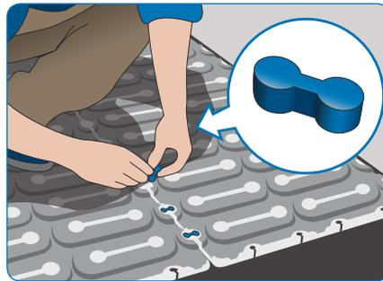
4) Install the Devicell™ Dry plates on the heated areas and optionally 13 mm plasterboards on the non-heated areas.
