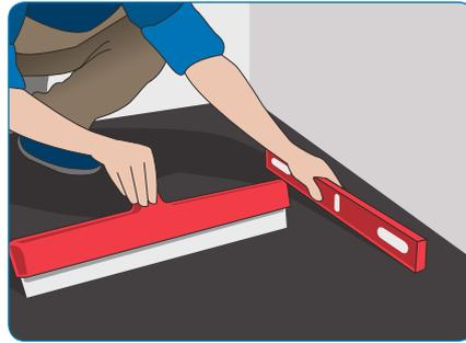
1) Make sure that the sub floor is reasonably level, firm and stable. New concrete needs to dry out for 30 days before installation.
