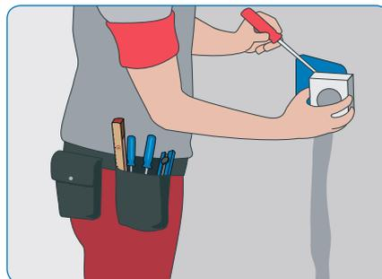
7) Check the insulation resistance and Ohm rating of the heating cables. Compare the Ohm rating with the nominal, written on the cable label. Plaster the wall groove and connect the cold tail, sensor and thermostat.
